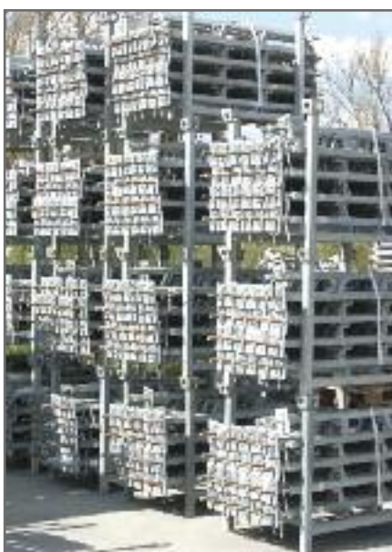
6 storing racks for railing posts can be stacked on a truck width. Up to 468 railing posts on a length of about 1.60 m.
