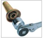
formwork the cones will be removed with the help of free wheel wrenches with hexagonal nut.
