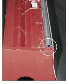
Usage of the profile "pine-tree" with ROBUSTA-round column formwork prevents the leaking of water and thus ugly grit spots. The result: prefab element quality at the in-situ-concrete construction site.
