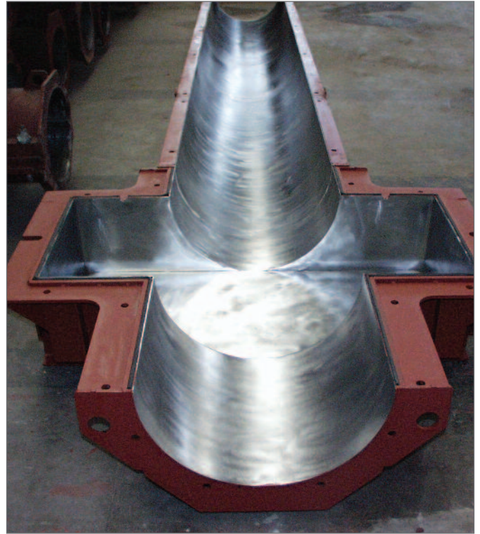
Formwork combined of rent and purchase parts for concreting at the prefab plant. Open round column formwork with a special attachment for 2 brackets.
