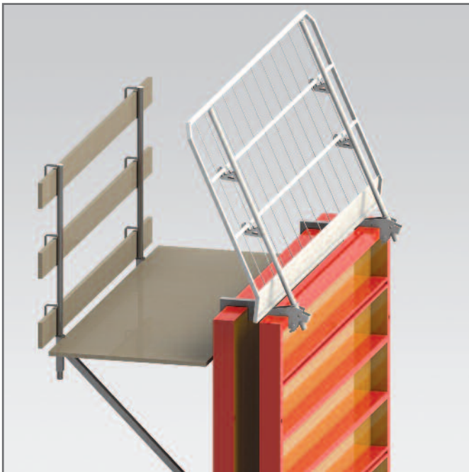
During mounting the railing posts and the boards are inclined towards the concreting platform.
