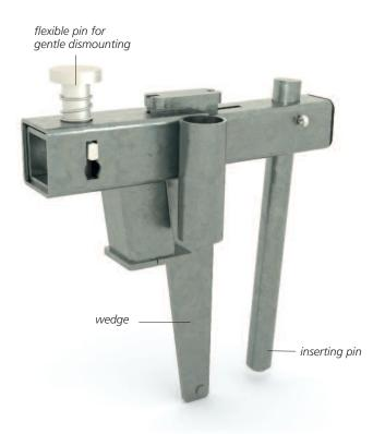
Because there are no cantilever parts, sealing and earthworks can be done without problems. With the flexible pin the clamp for twin walls can be adjusted for 6 and 8 cm thick cases and be removed quickly.
