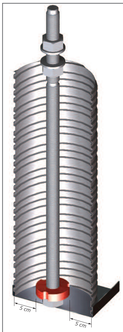
If the anchor plate is adjoining the tube, the grout will entirely enclose the plate due to the indents.
