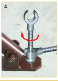
4. Final tightening of the screw by simply turning it with second screw-in set. Because of the form of a screw spanner of the screw-in set also a conical flange nut can be tightened.
