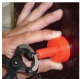
An easy removing oft the nailing flange by the double headed nail
