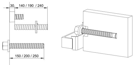
Installation-kit with **recoverable clamping flange** 30 mm, with bolt with suspension cone  $\emptyset$  26.5 mm **Sleeve length = bolt length –10 mm**
